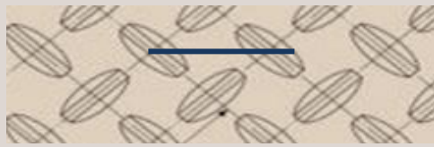
Teardrop pattern acc. ASTM A 786
